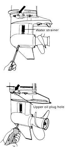
2) Insert the oil tube nozzle into the lower oil plug hole, and fill with gear oil by squeezing the oil tube until oil flows out of the upper plug hole.
