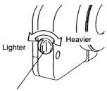
Throttle friction adjustment screw
