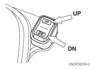
It is possible to tilt up or down in spite of main switch "ON" or "OFF".
