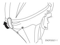
2. Remove starter lock cable from recoil starter by loosening the screw for the starter lock cable.
