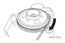
Tie a loop in the another end of the emergency starter rope and attach socket wrench that is included in the tool kit.
